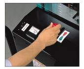
Easy Lifting and Lowering Lifting and lowering speed can be controlled by the operation of lever.
